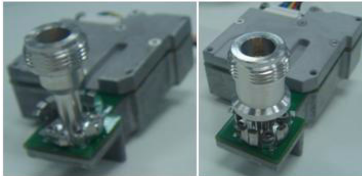
Figure 4-16 Calibrator assembly and improved calibrator assembly
